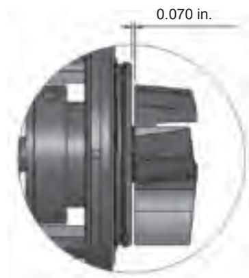
Figure A Spacing of the Impeller and Stub Shaft
